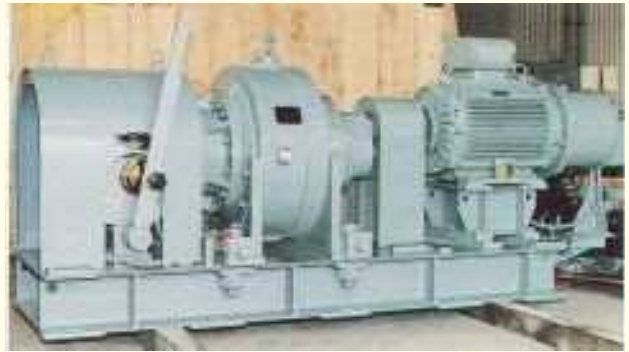
Inching Device for Cement Mill
